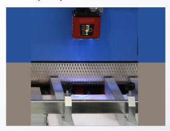
The Sequence Control System is carried out by an OMRON camera.
