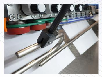
The **New Roller Guide** presses each single folded sheet to achieve excellent quality folded signatures before sewing. Springy sheet transport rollers allow the system to adapt to sheet thickness with improved control and fine adjustment.
