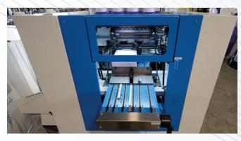
Sewn book blocks are delivered spine-up onto a compactly-designed **delivery table** for easy unloading.
