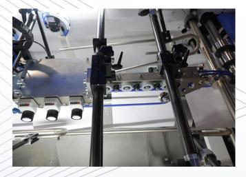
The **Sheet Plow Folding** Station cross-folds the sheets into "four pages". After folding, each single sheet is driven inside the new pressing roller guides. Sheet transport pulleys are equipped with a fine adjustable system to cater to different paper types and increase / decrease the friction between the transport polycord belt and the sheets.
