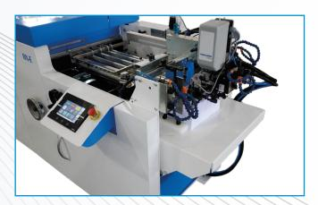
**Smyth pile feeder** supplied complete with self-positioning head, vacuum separation system, and suction wheel for sheet feeding.
