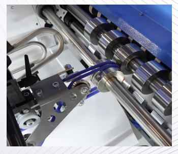
Two slitter shafts guide each single sheet into the Scoring Station. Here the special Tech-ni-Fold Tri-Creaser Fast Fit device guarantees the highest possible quality creasing and folding, including landscape format.
