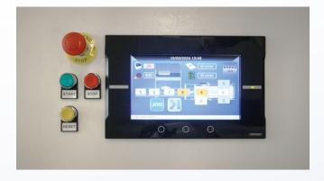
The **operator interface** comprises a touch screen to enable all machine operating and book program parameters.
