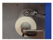
Both upper and lower mandrels have a hinged support and the lower mandrel has a perforator mounted above it to aid separation.
