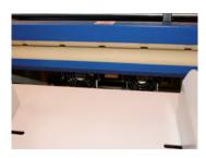
The electronically adjustable burster automatically separates sheets up to B3 size whilst fans provide a cushion of air to support the sheet as it is delivered into the catch tray.
