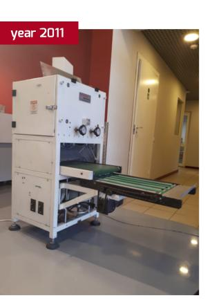
An effective and easy to use book press and creasing machine. One operator can operate the machine while operating the SCI-L Casing-in Machine.
