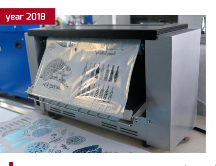
The DC-2 Dry Coater and Foiler provides a quick solution that enhances the value and vibrancy of any toner based digitally printed pieces to give them instantly, a glossy, foily and shiny effect.
