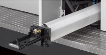
Automatic impression cylinder cleaning*
